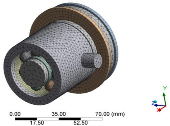
Figure 7: FE model for multi-blade rotary friction tool
