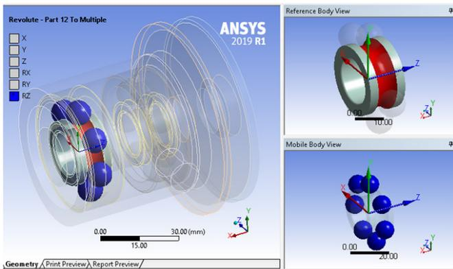
Figure 6: Setting up the bearing unit connection
