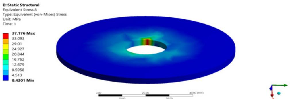
Figure 9: Stress state of the cutting cupped cutter
