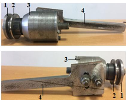
Figure 1: Multi-blade rotary friction tool: 1-heating cupped cutter; 2-cutting cupped cutter; 3-shell; 4-holder
