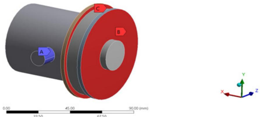
Figure 8: Boundary conditions of a multi-blade rotary friction tool
