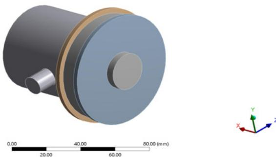
Figure 2: Three-Dimensional model of the body of a multi-blade rotary friction tool
