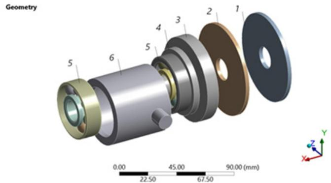
Figure 3: Nodes of multi-blade rotary friction tool: 1-heating cupped cutter, 2 - cutting cupped cutter, 3-sleeve, 4-shaft, 5-radial thrust bearing, 6-shell
